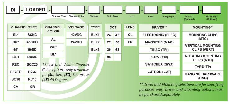
Example: DI-LOADED-SQBL-24V-BLX3-CL-36-CV = Diode LED, Fully Loaded, Square, Black Channel, 24 Volt, BLAZE™ X 300, Clear Lens, 36 inches , 96" Lead Wire, and with a Constant Voltage Driver.
