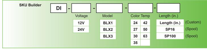
*Example: DI-12V-BLX3-27-SP16 = Diode LED, 12 Volt, BLAZE™ X, Type 3, 2,700° CCT, 16.4' spool.*
