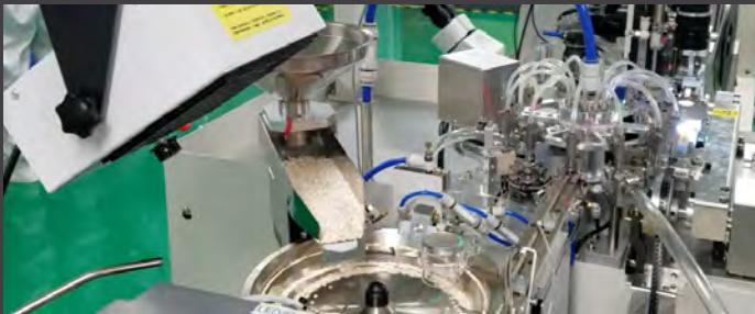
SORTING & BINNING. Each LED chip is sorted and measured by high-precision cameras and computer systems to collect LEDs into batches for accuracy of Correlated Color Temperature (CCT) and Color Rendering Index (CRI) measurements.
