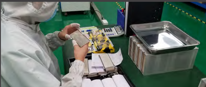
QUALITY CHECK. LEDs are inspected by engineers for physical or electrical flaws and irregularities before the sorting process begins.
