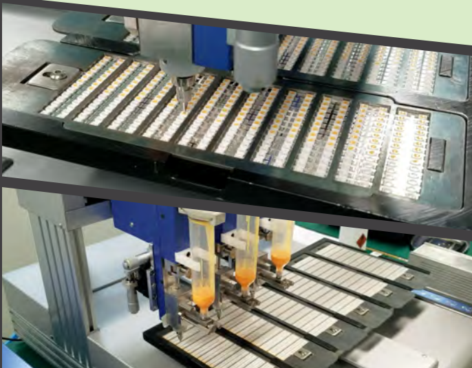
PHOSPHOR APPLICATION. Phosphor Injection creates the most precise photometric output with state-of-the-art technology and yields less waste than traditional spray-coat methods.
